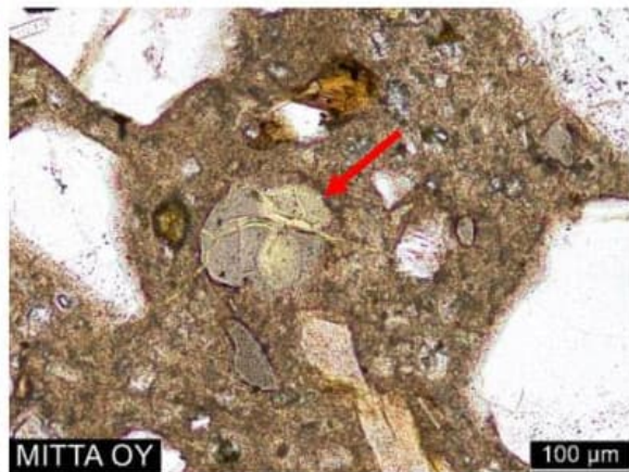
Figure 32. Cracking has proceeded to the paste from the silica fume lump. PPL
