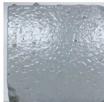
B5/L8 – Epoxy coating
