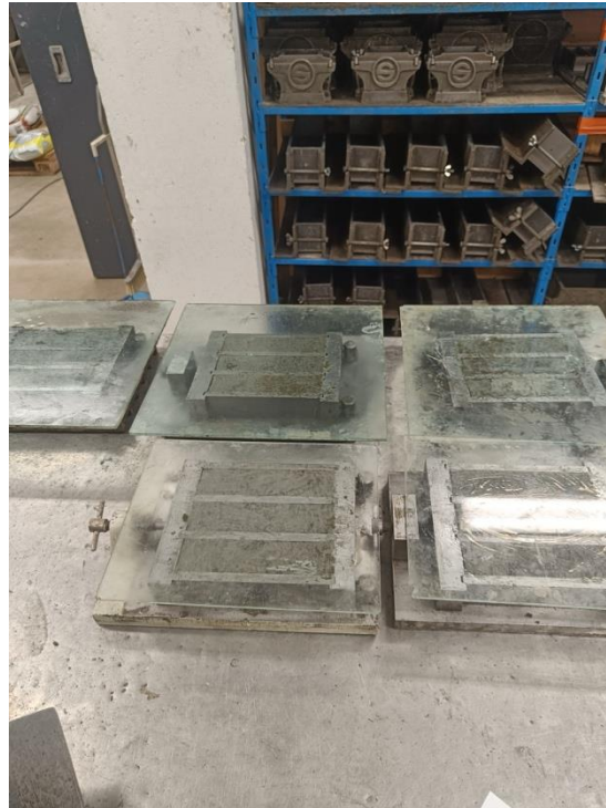
Figure 2: Moulds covered with glass, to have a smoother casting surface.
