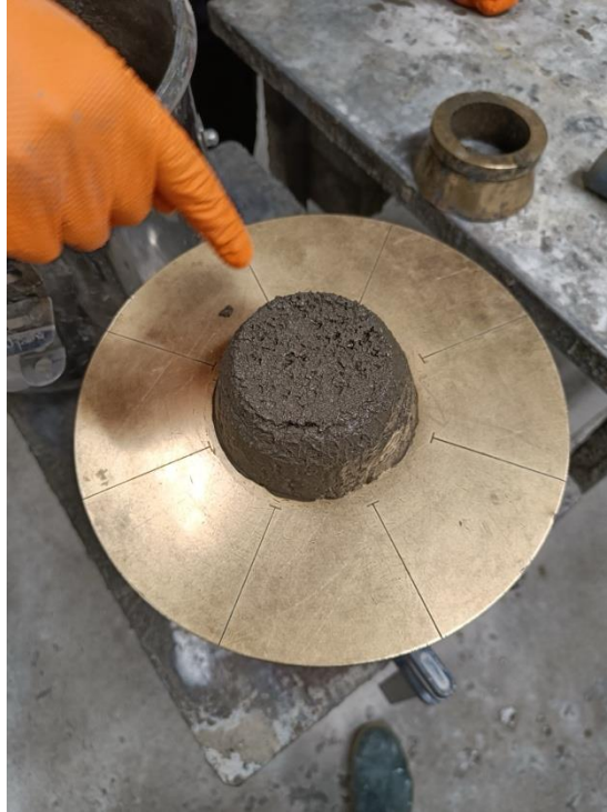
Figure 6: Mortar slump flow test (before compaction).
