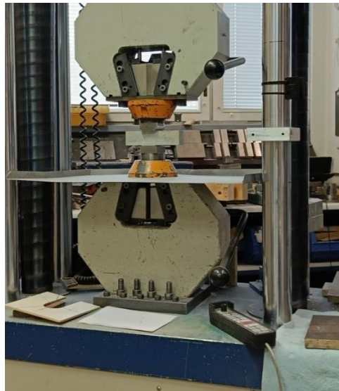
Figure 10: Initial compressive strength test of a mortar specimen.
