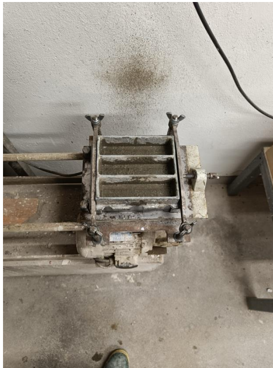
Figure 1: Mould filling and compaction of the specimens.
