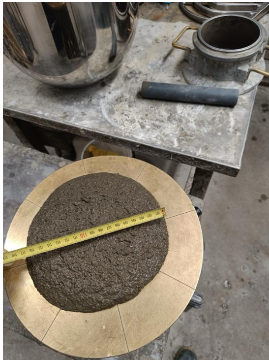
Figure 7: Mortar slump flow test (after compaction + result).
