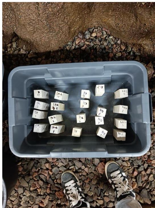
Figure 5: Storage container for the sulfate attack investigation.
