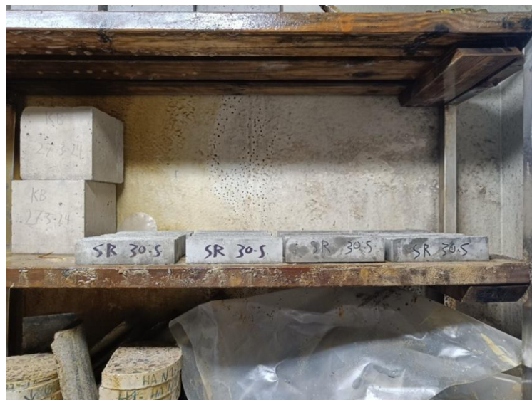
Figure 3: Specimens placed in the 95% humidity chamber.
