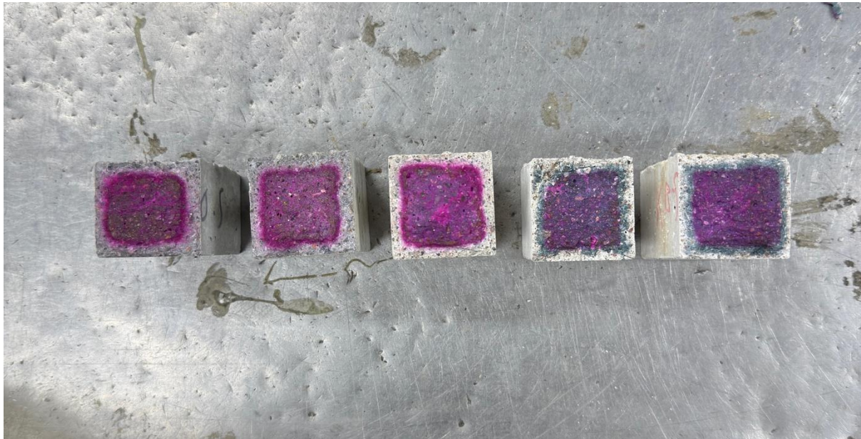
Figure 11: Phenolphthalein test in the mortar mixes.
