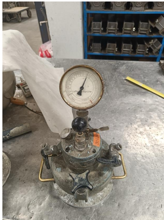
Figure 8: Pressurized air content measurement device (1 litre).
