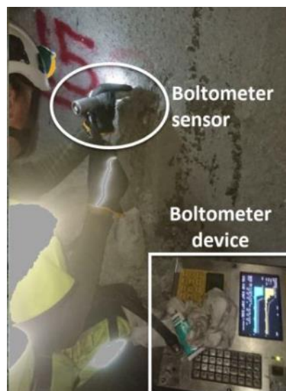
Figure 23. NDT of rock bolts by the use of guided ultrasonic waves: The Boltometer [19].
