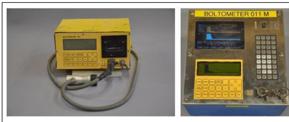
Figure 15. Boltometer instruments for non-destructive testing of rock bolt embedment [19].
