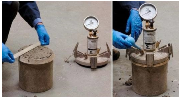
Figure 9. Determination of Air Content in Fresh Concrete: Pressure gauge method.
