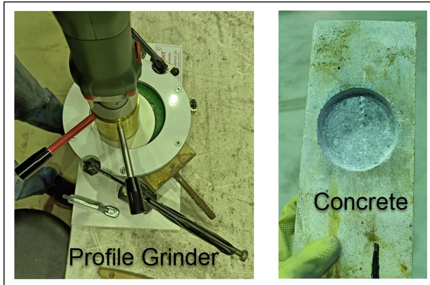
Figure 27. Concrete sampling for chloride measurement – Profile grinder.
