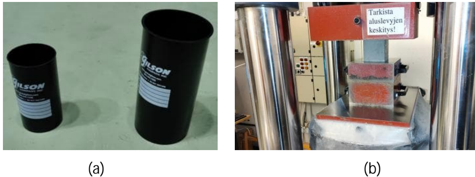
Figure 12. (a) Moulds for the two standard sizes of concrete test cylinders and (b) compression test machine.
