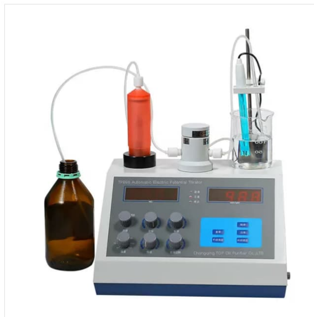
Figure 26. Example of the potentiometric titrators used in the titration method.
