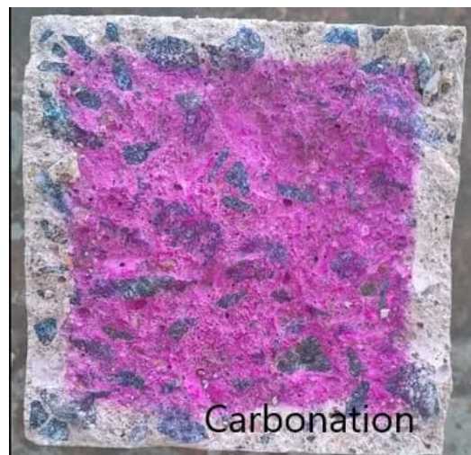
Figure 15: Carbonation testing of a concrete specimen.
