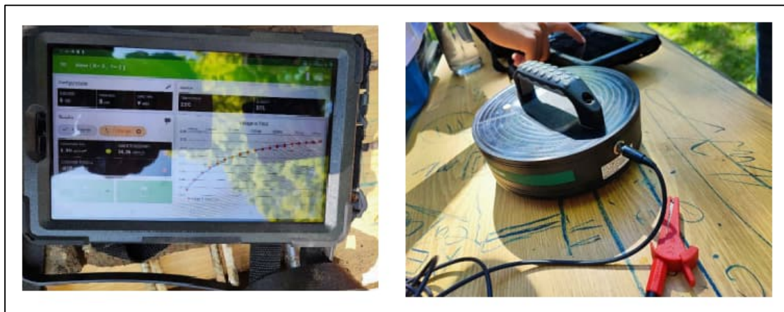
Figure 25. Example of using the iCor device for measuring the electrochemical corrosion of steel.
