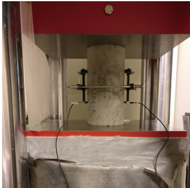
Figure 16. modulus of elasticity in compression test of hardened concrete test (Photo: Jukka Piironen).
