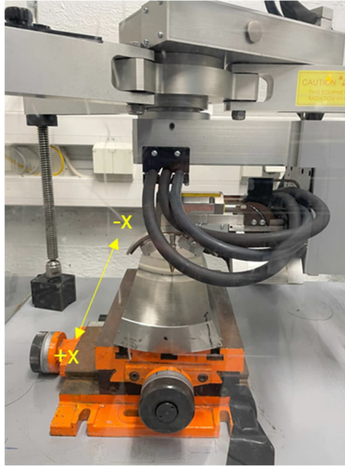
Figure 2. Residual stress measurement setup.
