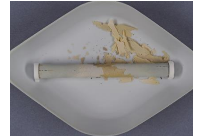
Post-test photos and optical micrograph of a cross-section cut from the middle part of the TiAl coated sample exposed for 5 minutes. This sample had no filling powder.
