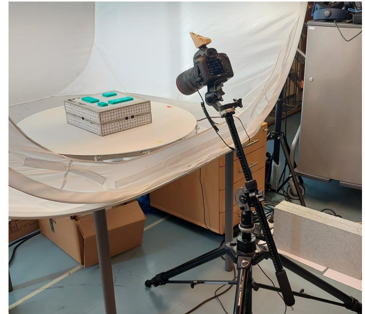
Close-range photogrammetry using a rotating table and a light-tent. Green ceramic calibration pieces can be seen on top of the Kury gray granite sample pair.
