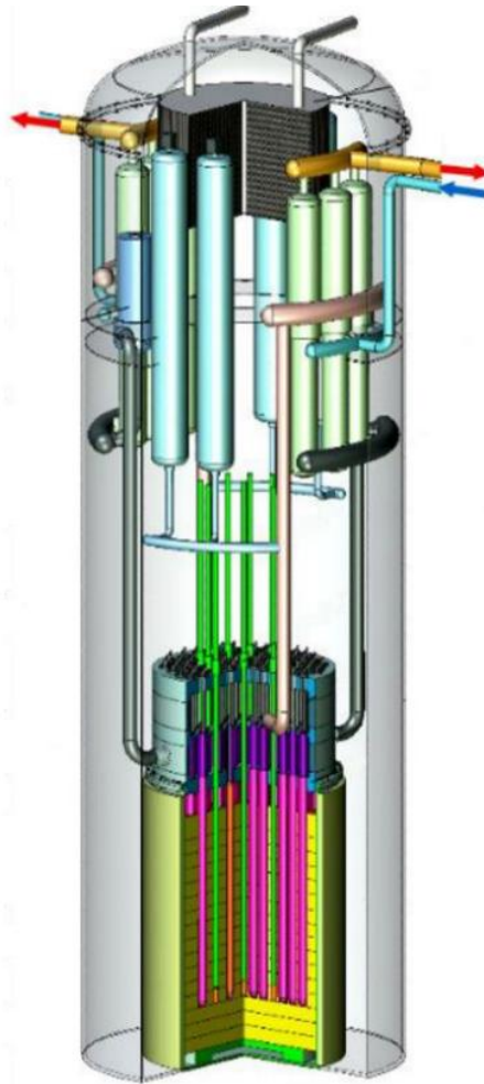
Figure 13. A schematic of Star Energy SA's STAR 10 MWe micro reactor. [10]
