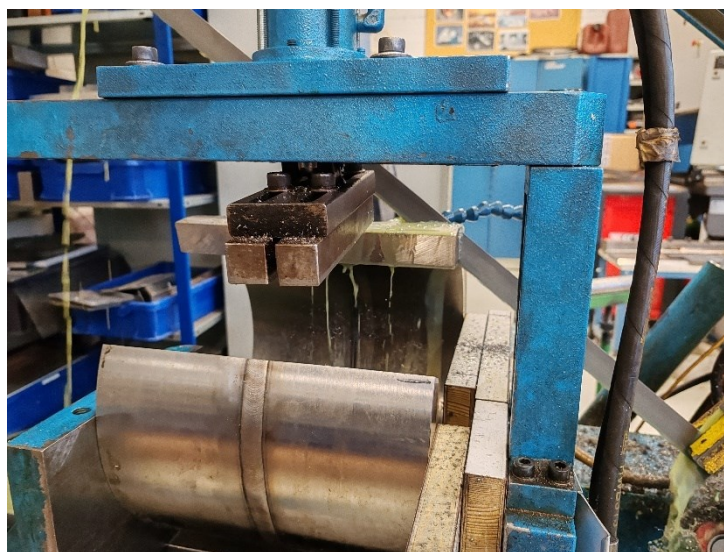
Figure 25 : Pipe cutting operation.
