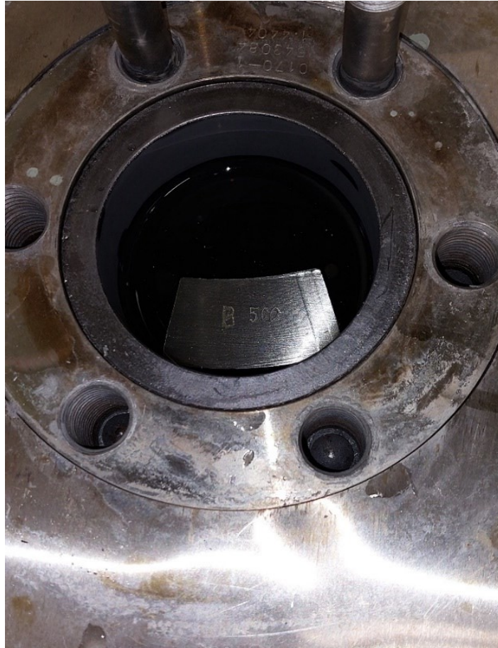
Figure 32 : Sample placement in the autoclaves for SCC test.
