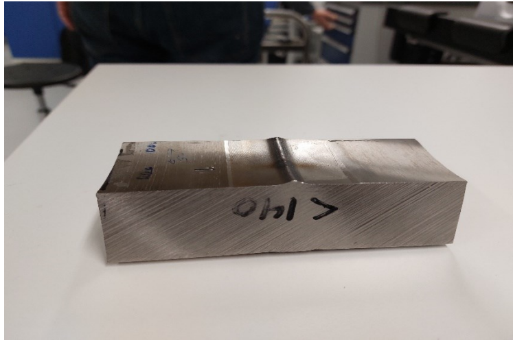
Figure 26 : As cut sample from the pipe ring.
