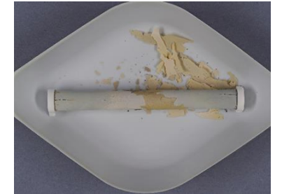
Post-test photos and optical micrograph of a cross-section cut from the middle part of the TiAl coated sample exposed for 5 minutes. This sample had no filling powder.
