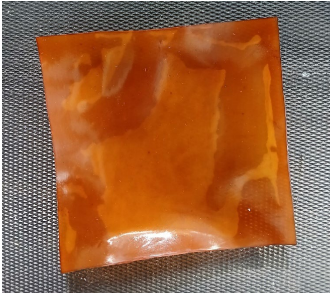
Figure 8. A XLPE sheet after the fast aging done inside an oven.
