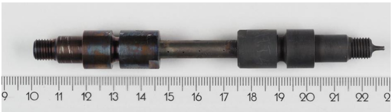
Figure 4. The mechanically plugged biaxial creep testing specimen
